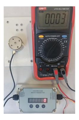
**2)** Long-press K1 to enter setting mode, short-press K1 to find "08\_\_CZ", to set transmitter zero point; long-press K2 to enter, make sure it is all zero, and check the multimeter reading is also zero or really close;
