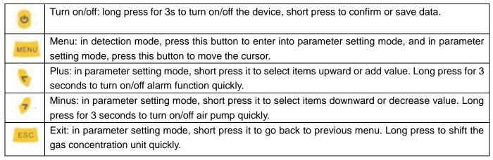
(Note: The long press function only work in detection mode. When you change or reset any data, please remember to click "ON/OFF" button to confirm and save the settings. Remember to turn on the pump when start the detection. Please turn off the pump when there is no need to detect, which will be helpful for the service life of the pump.)
