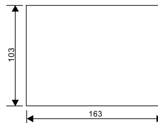
Panel cutting dimensions for panel mounting
