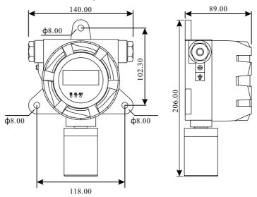
• Apperance and installation hole map of gas detector with alarm light
