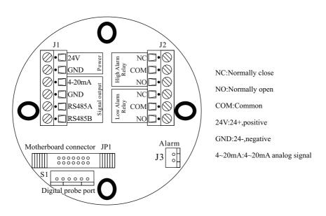
Note: Do not connect wires with power on at any time.
