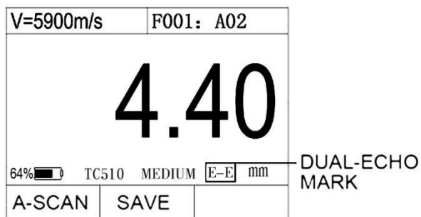
Figure3.9 THICKNESS MEASUREMENT INTERFACE WITH THROUGH COATING MODE
