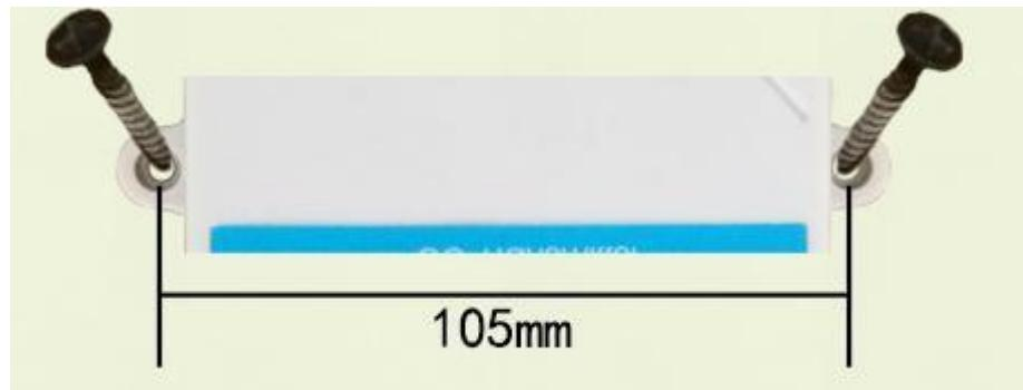
Wall-mounted installation. Mounting holes are located at the center of both sides of the device. The hole diameter is less than 4mm, with a hole spacing of 105mm. Installation can be performed using 3mm self-tapping screws.
