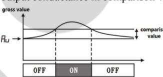
$LP-S$  indicates positive deviation between gross value and given value  $RU >$  the output conductance in comparison value
