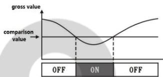
$HP-S$  indicates positive deviation between gross value and given value  $RU >$  the output conductance in comparison value
