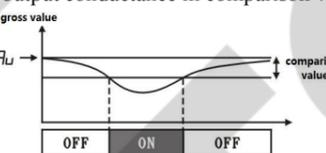
$HLPS$  indicates the deviation absolute value of gross value and set value  $RU >$  the output conductance in comparison value
