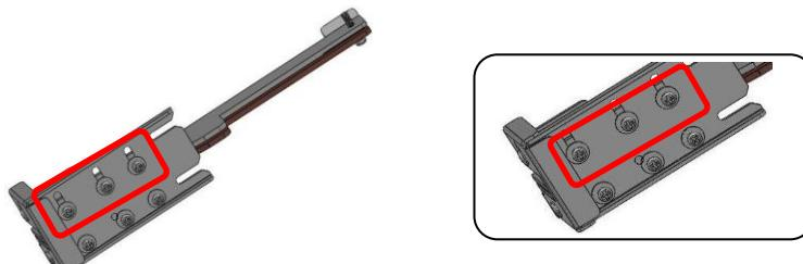
6. Loosen the screw fastening the Tooling Plates at the rear end of Rail Assembly, take out the screw and the Tooling Plate.
