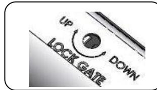
2. Same to loosen the screw in the Lock Gate hole (between UP-DOWN) at right side Housing plate.
