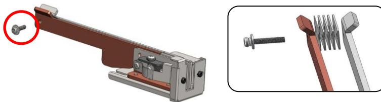
7. Refer to the following table, select the Front Tooling Plate (0.8mm, 1.0mm, 1.2mm, 1.5mm, 2.0mm) and insert it into the front Rail Groove for the width required and tighten the screws in the long-circular holes (reverse of step 4 & 5).
