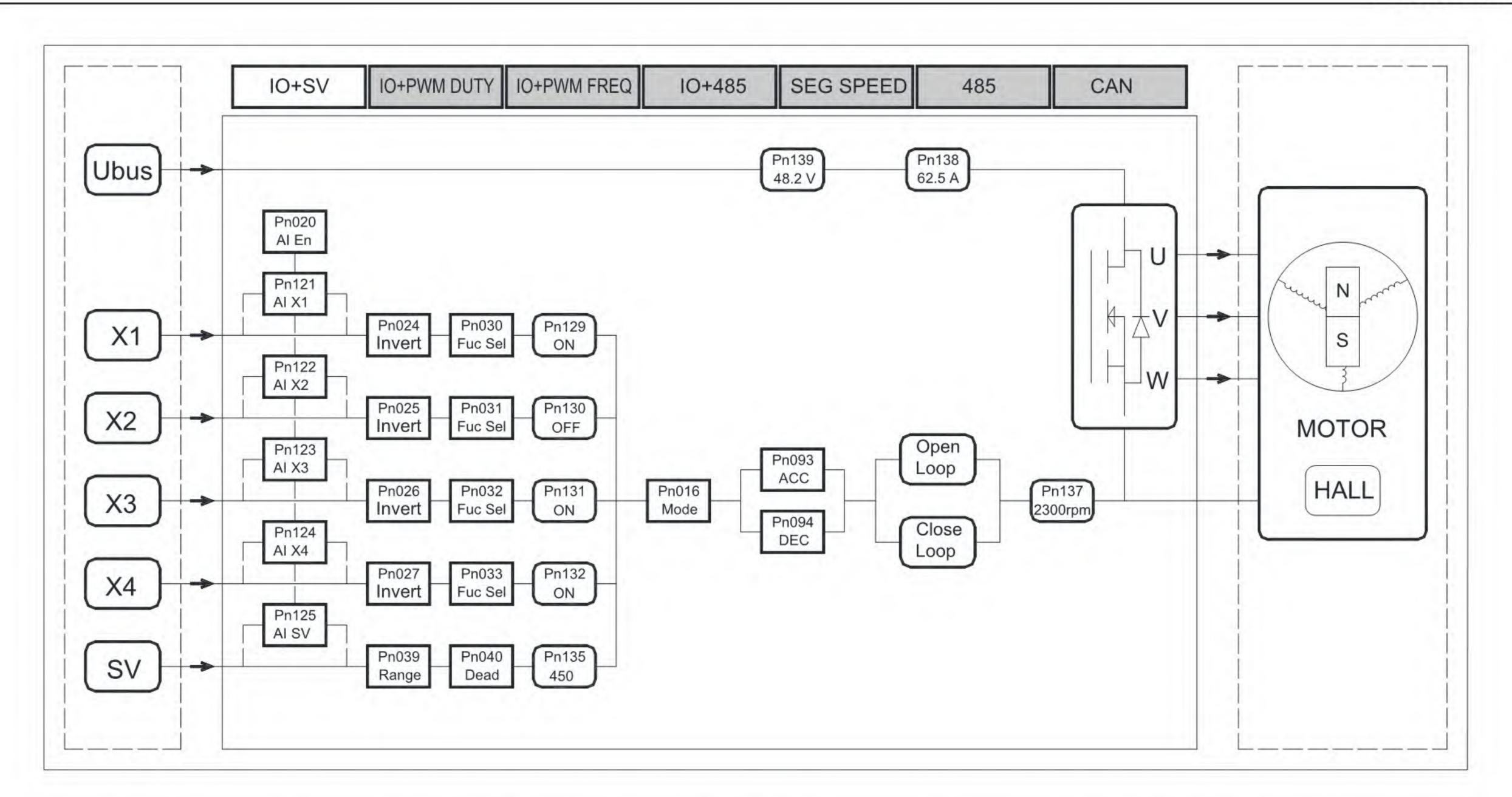
In this control mode, the switching inputs of X1~X4 are used as motor start/stop, brake and direction change control.
