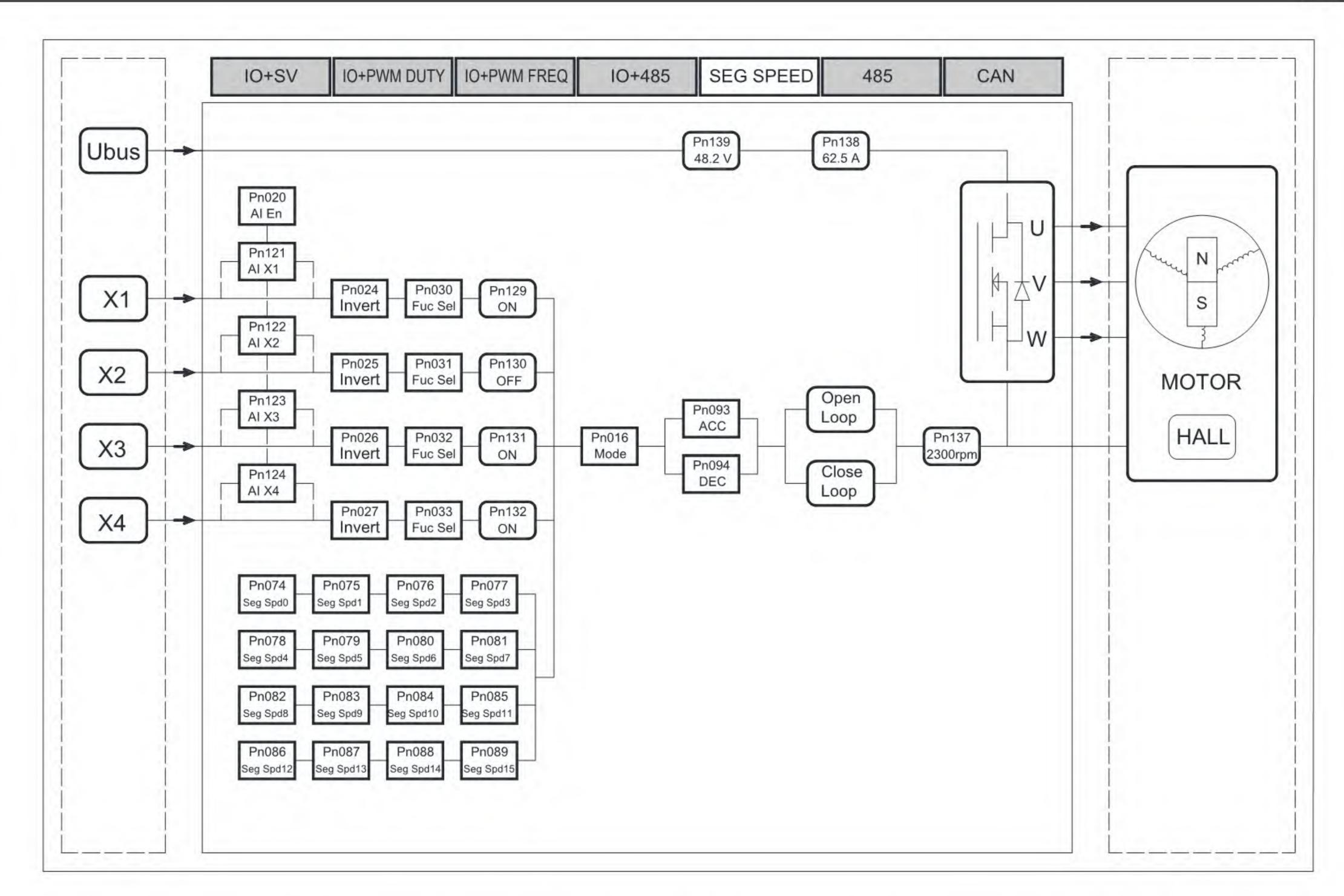
In this control mode, the switching inputs of X1~X4 are used as the control inputs for segment speeds, and the 16 states of the 4 inputs correspond to the 16 speeds in the parameters Pn074~Pn089 respectively.
