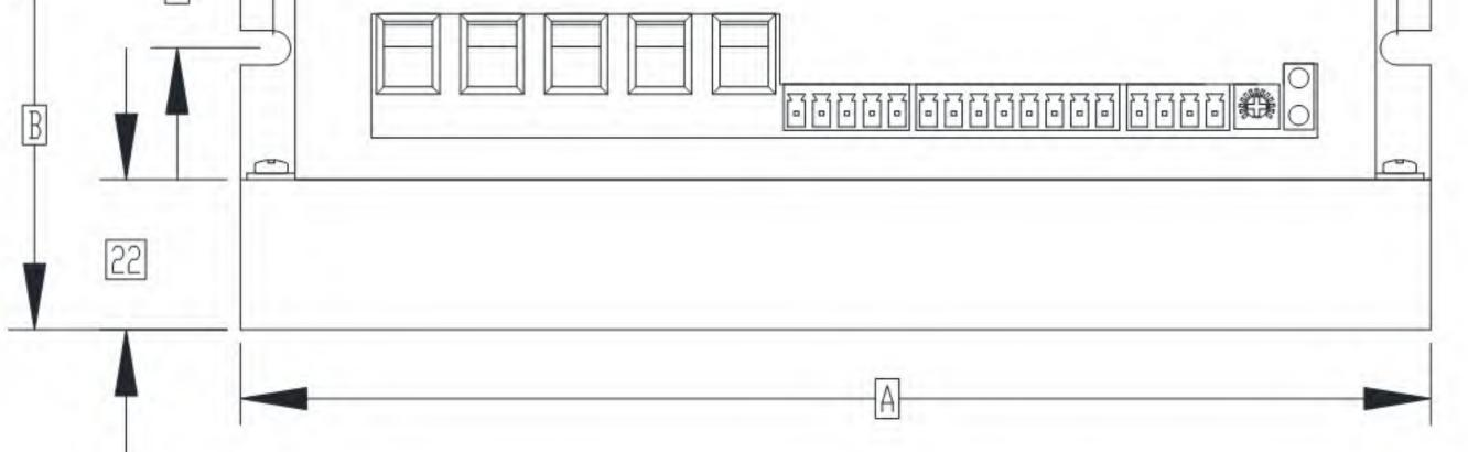
Fixing Screws: 2\*M8, recommended locking torque: 0.55N.m.
