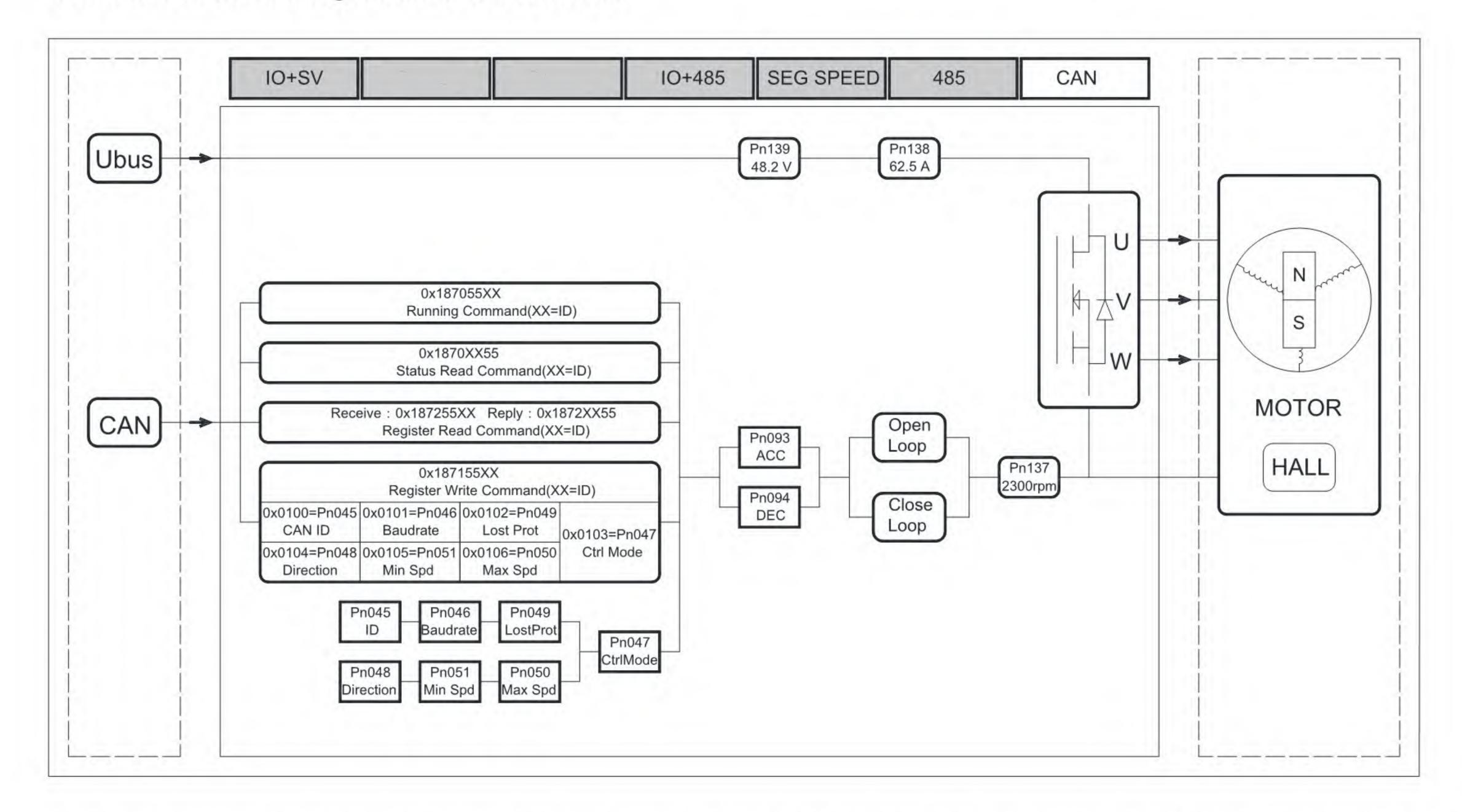
In this control mode, the control of the system can be realized only through the CAN communication port, and the communication protocol is customized CAN protocol.
