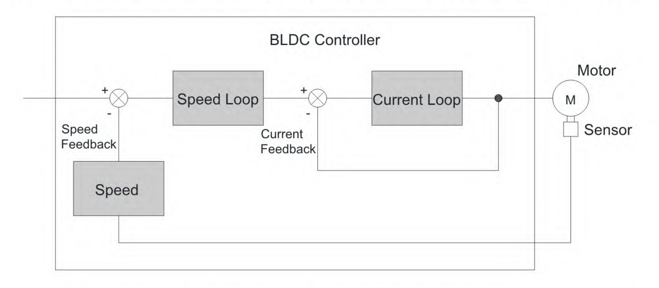
The driver is the control core of the DC brushless control system. By processing the input signal and feedback signal, the brushless driver can provide accurate speed and torque control of the brushless motor, i.e., speed and torque control mode. Among them, speed control is the most important and commonly used control mode of the system.
