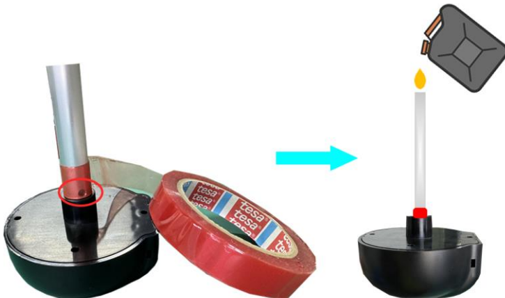
Closing the drain holes, rotating the sensor, and filling the tubes with fuel
