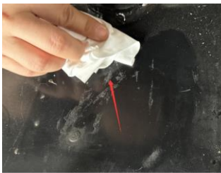
Clean the installation position of the oil sensor and remove dust and dirt from the surface of the fuel tank
