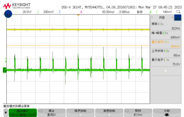
Figure 9, Short circuit & Output voltage
