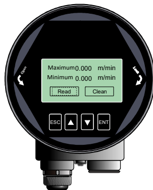
Figure 6-15 Historical Emptying Rate Display Interface
