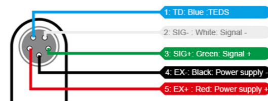
Figure 2-7 Internal wiring diagram
