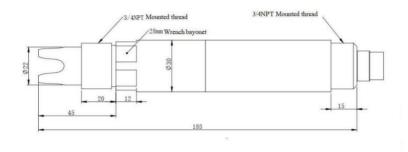
Note: The sensor connector is M16-5 core waterproof joint male head.
