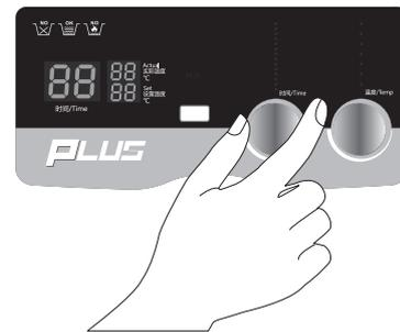
PLUS series: At first setting, the time is random, progress bar light on, turn the rotary knob clockwise to increase time. Turn counterclockwise to decrease time. Correspondingly the two digits on the left of the display change accordingly, and the time setting done well. Press the rotary knob, ultrasonic start working.
