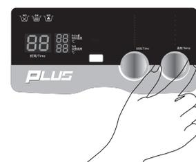
S series: At first setting, the temperature is random. Touch "Temp+" or "Temp-" to increase or decrease temperature. Press "on/Off" button heat will active before reaching the setup temperature.
