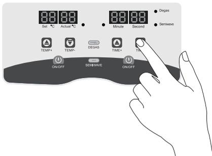
S series: At first setting, the time is random. Touch "Time+" or "Time-" to set time, press "On/off" the ultrasonic active and the machine start to countdown.
