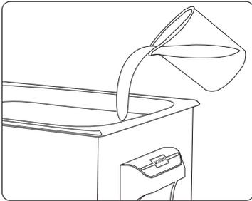
Fill the tank with warm or tap water below the maxline; Add required quantity of cleaning solution. When using flammable liquid such as alcohol, gasoline and so on, heating is strictly forbidden! Ultrasonic vibration for a long time cause temperature of liquid increase, caution fire.
