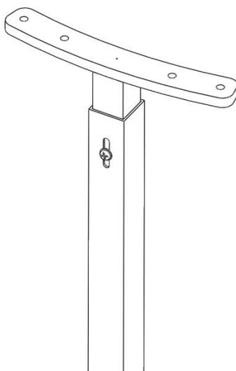
Attach the three windshield retaining rings to the three windshield support brackets using M5 wing screws (M5\*16).
