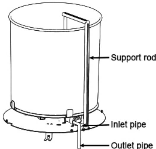
After installation is complete, reinstall the outer casing onto the base.
