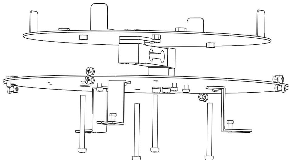
Screw the three leveling bolts (M5\*10) into the base plate. Place the entire base plate onto the foundation. Secure the base plate to the foundation using three sets of fixing bolts (M8\*20) and nuts (M8) (do not fully tighten the bolts). Adjust the three leveling bolts until the base plate is level with the foundation surface. Then, use a wrench to fully tighten the three sets of fixing bolts. Connect the heating device plug to the main control unit.
